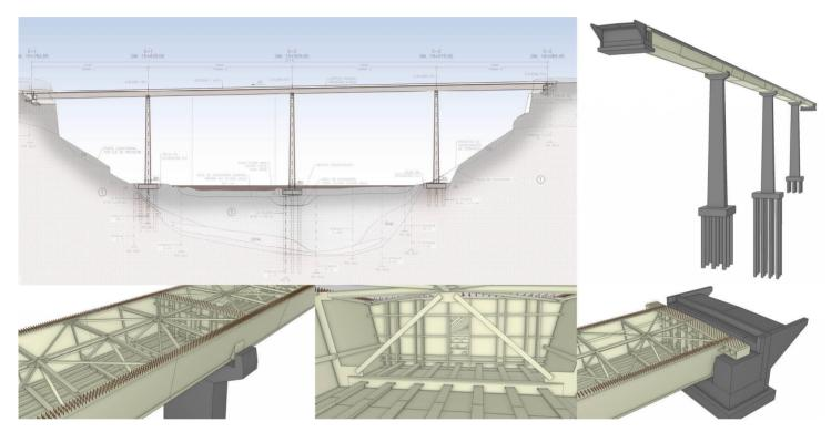
The Yalquincha viaduct is a 318 m long composite box girder bridge with four spans of 70.5, 90.0, 90.0 y 67.5 m. Thje bridge is part of the Calama bypass, which is part of the Rutas del Loa PPP project.
